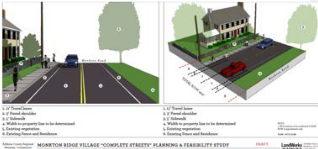
Graphics from Monkton Complete Street Study showing alternative street designs for safer streets.
